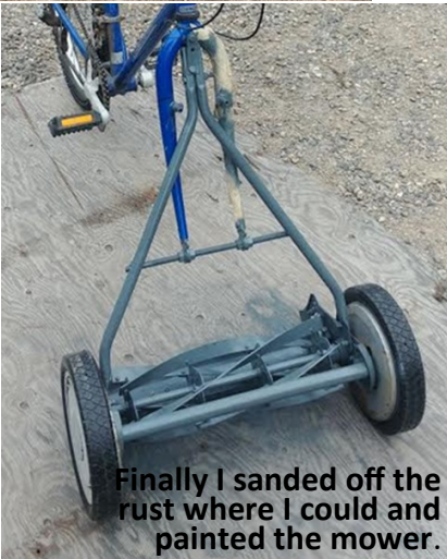
My Dad TIG (tungsten inert gas) welded the mower to the bolt attached to the bike. It was pretty tricky to weld, since the bolt was way thicker than the tubing on the mower.
