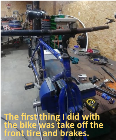
Next I put on some newer handlebars I had laying around. Then I put a bolt where the bike tire, axle and hub were; I used some nuts and locked them to all sides of the fork to hold the bolt in place.
