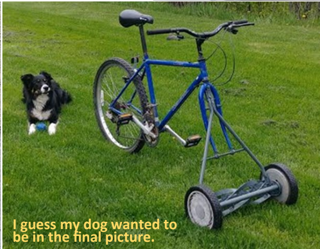
The first thing I did with the bike was take off the front tire and brakes.
